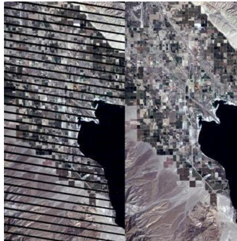
Scan Line Corrector Malfunction
